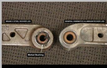
Operating at 1.45 in. stroke, the steel rocker leg on the left caused the bushing to fail due to over heating, while the GK aluminum leg dissipated the increased heat and continued to run flawlessly.
