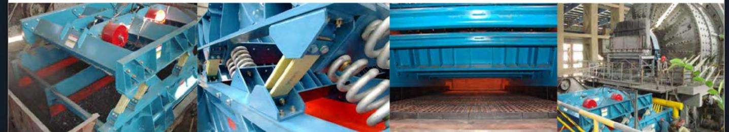
STM-S™ single deck and STM-D™ dual deck series of vibrating screens utilize GK's proven two-mass / sub-natural frequency drive design which uses up to 75% less horsepower than conventional screen designs, significantly reducing energy consumption and cost.
