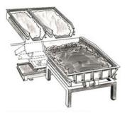
With GK's Charge Make-up Solutions, materials are loaded into either vibratory feeders or stationary bin with clam-shell bottom gates. Both options are mounted on weigh cells to determine the weight of charge material.
