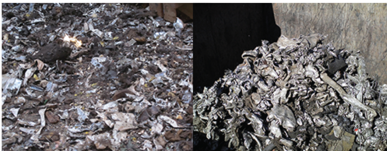
Material before the DE-STONER ® Material after the DE-STONER ®
